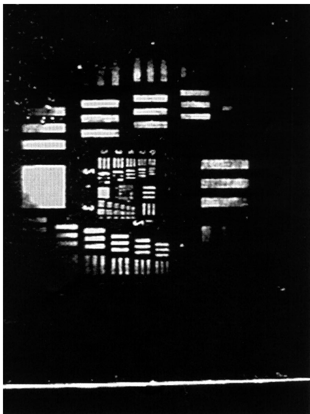
Fig. 5 USAF Resolution target image written in 9-decylantracene photodimer-PMMA. Stored by two-photon excitation using 532 nm pulses. Accessing by a single, 370 nm, photon process.
